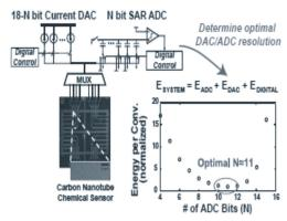
Fig. 5. Block diagram of a carbon nanotube chemical sensing system [18].
