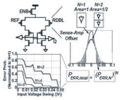
Fig. 4. Redundancy significantly reduces the error probability in the SRAM sensing network [13].
